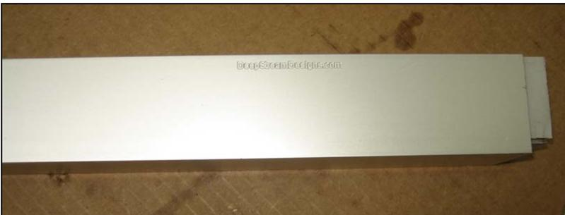
Detail of 7-year old proprietary marine anodized leg, near flawless with no deterioration.
